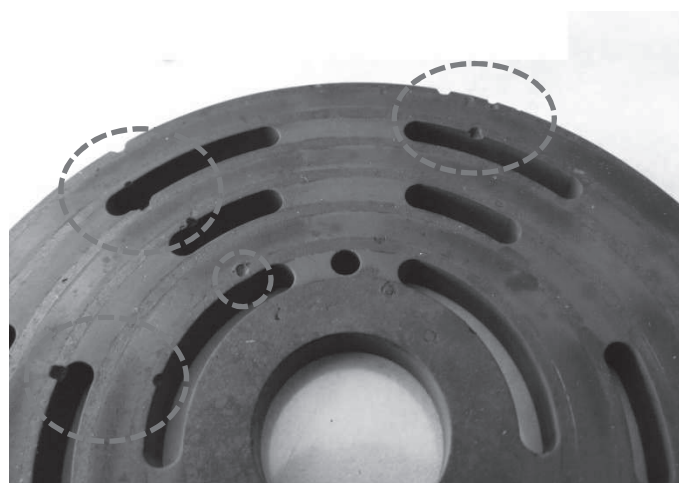
Figure 2 – Example of damaged valve plate by external elements
