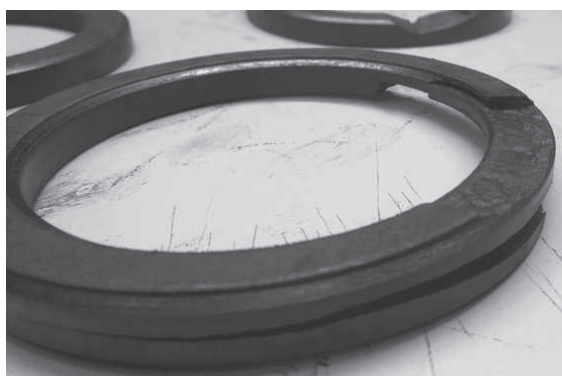
Figure 9. Valve ring damages observed on individual rings of the multi-ring valve.
