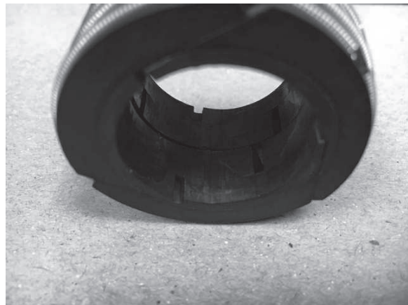
Figure 5 – Overheated AL Ring
