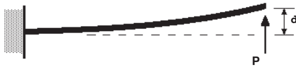
Figure A.1 Deflection of a Cantilever Beam due to an applied Force
