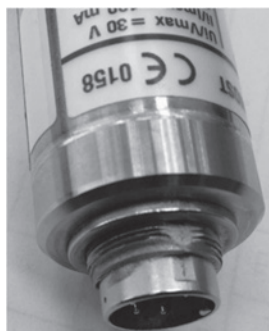
a) b) Figure 3: a) Shows the sensor cable connection socket with thread damage b) Cable connection socket with heavy corrosion
