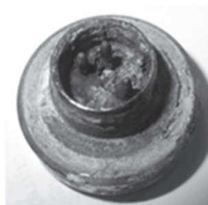
a) b) Figure 3: a) Shows the sensor cable connection socket with thread damage b) Cable connection socket with heavy corrosion
