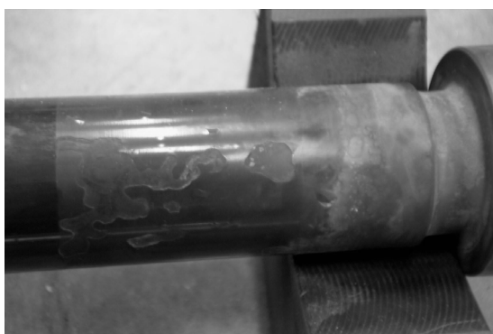
Picture 3: Underlayer corrosion on oxide coated NH 3 piston rod
