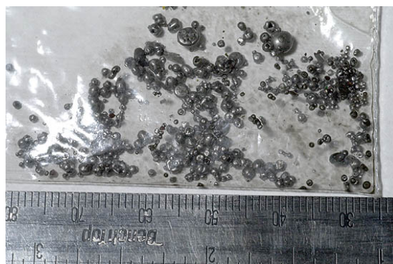
Picture 18. Debris removed from Compressor Gas Piping
