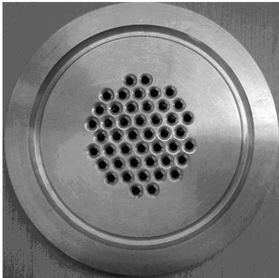
Fig. 9: Gas inlet side of patented “pulsation damper plate based on the KÖTTER principle” fitted to cylinder output flange of second stage.
