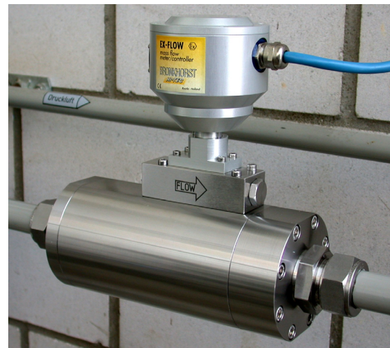
Fig. 6: Measurement of hydrogen flow rate by means of a thermal mass flowmeter for potentially explosive atmospheres
