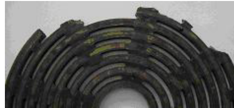
Figure 2: Impact failure of a valve plate caused by sticktion.
