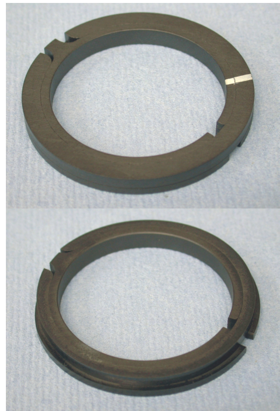
Fig. 4: Unequal wear of cover ring and sealing ring made of high-temperature polymer (bottom), compared with a new twin ring (top)
