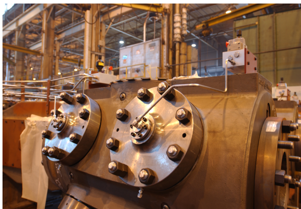
Picture 13. – BOS Compressor Cylinder with D-R ISC Mounted (Note: Only One Solenoid is Required per End for Compressor Valves)
