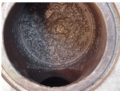
Fig. 3: Erosion damage behind the suction nozzle of the fourth stage
