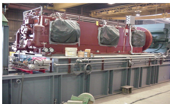
Picture 19. BOS Compressor Mounted on a Compressor Skid complete with Electric Motor
