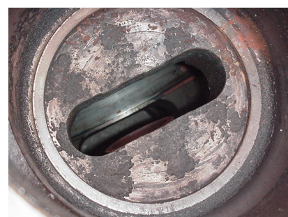
Fig. 5: Erosion damage at suction valve seat
