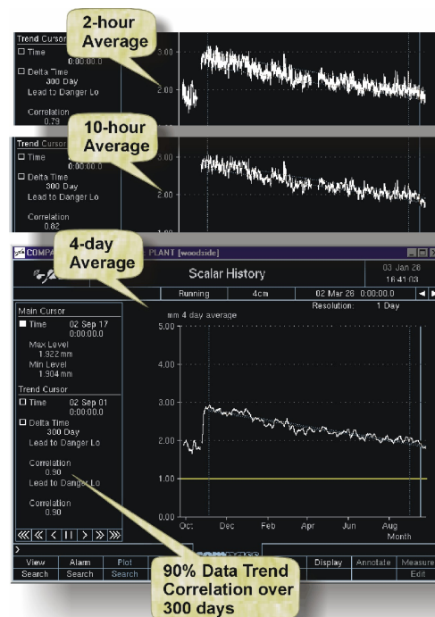
Fig. 5 Different averaging routines are done simultaneously on the same rod drop measurement. The 4-day average can establish a good long-term trend. The non-averaged measurement is important for catching short-term faults such as the lubrication fault shown in Fig. 6 or the sand-in-the-cylinder problem shown in Fig 7.
