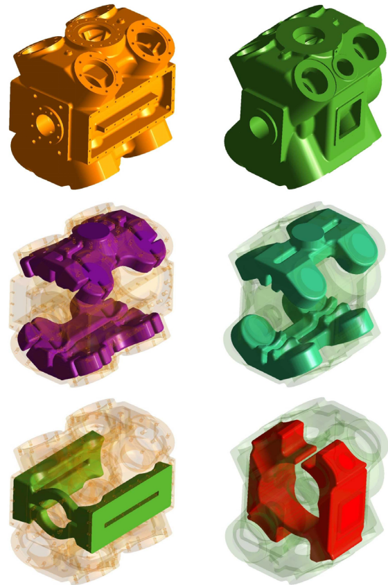
Figure 4.1.11: Comparison of standard (left side) and new (right side) cylinder design - complete cylinder (top), discharge/suction gas chamber (middle), cooling water cavities (bottom)
