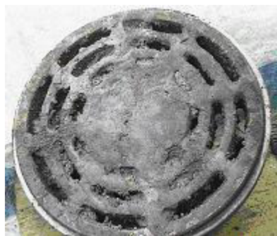
Figure 1: Fouling of a compressor valve.
