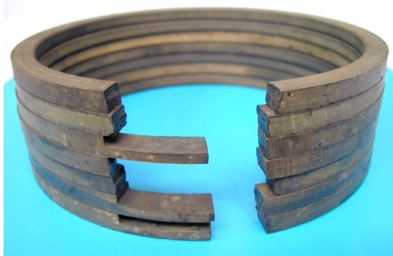
Fig. 2: Step-cut piston rings made of a brittle polymer blend and exhibiting fracture of the overlapping joints
