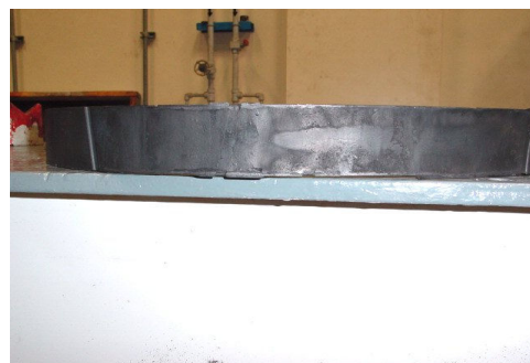
Fig 15: Heated effected Rider Rings
