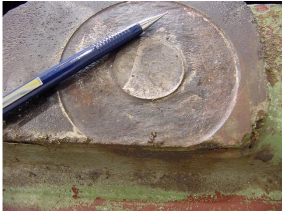
(Picture 2.1.3: Frame Bottom Hammering Marks)
