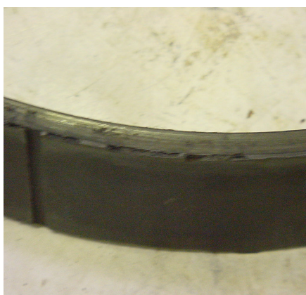
Fig 12: Chipped off material from Rider ring of 1 st stage
