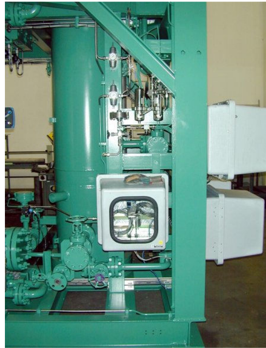
Figure 3: Condensate drain system of a process gas compressor unit
