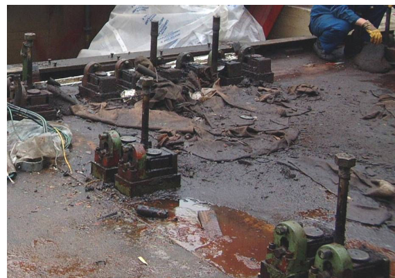
(Picture 2.3.1: Support Blocks in bad Condition)
