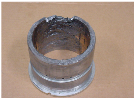
Fig 8: Crosshead Bearing damaged
