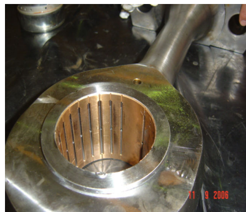
Fig 11: Unloaded side remain intact
