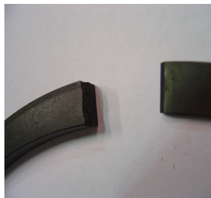
Fig 13: Piston ring broke off from overlap portions
