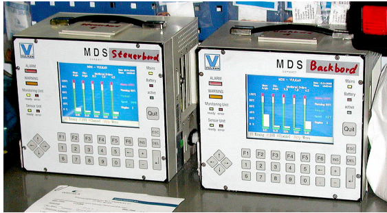
Figure 6: Two continuous monitoring devices used for engine and flexible coupling control
