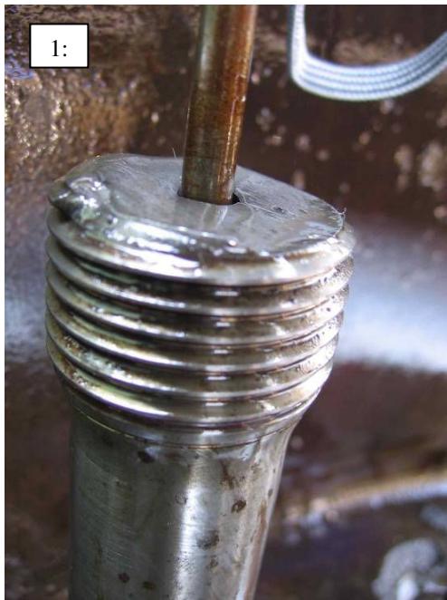
(Picture 2.4.6: Fractured Bolt Surface)
