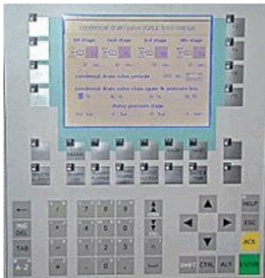
Figure 4: Human machine interface for the manual condensate drain adjustment
