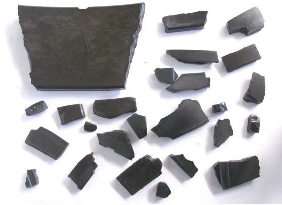
Figure 11: Damage to rider rings resulting from high temperatures during dry-running under unfavourable tribological conditions
