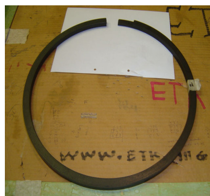
Fig 14: 1 st Piston ring with one overlap portion intact
