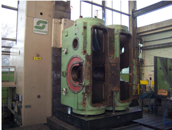
(Picture 3.1.1: Hyper Frame on Milling Machine)
