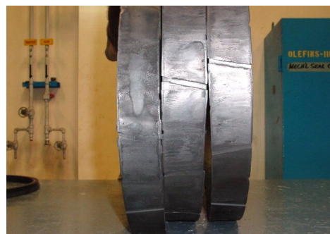
Fig 16: Set of rider ring effected due to high temperature
