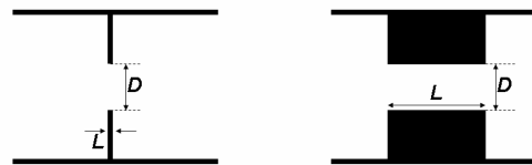
Figure 4: Thin and thick orifice configurations
