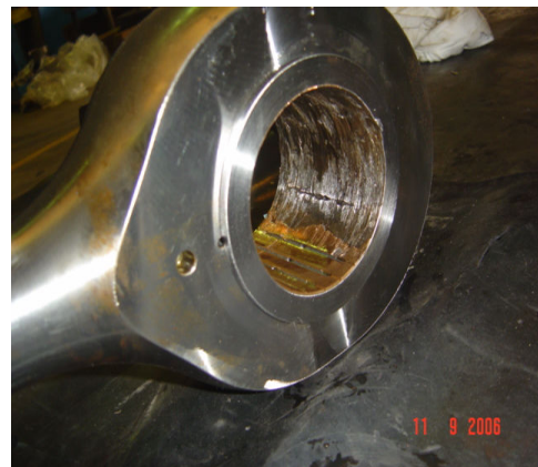
Fig 10: Connecting rod small-end damage
