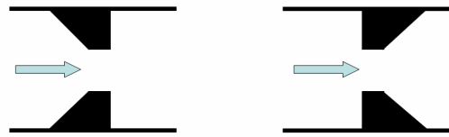
Figure 6: Orifice with beveled upstream and downstream edges
