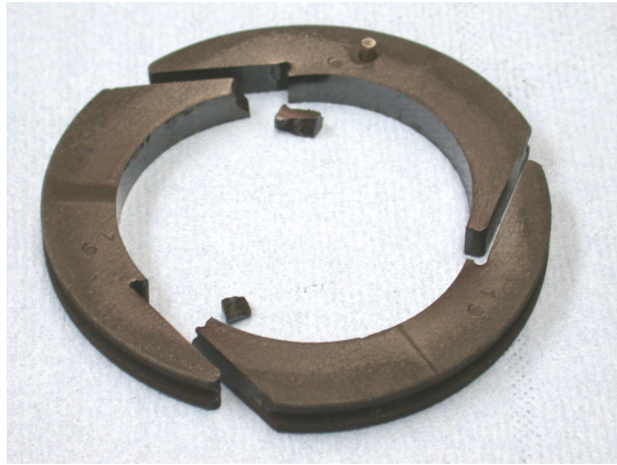
Figure 5: Plastic deformation and damage to a packing ring caused by high temperatures resulting from inadequate piston-rod roughness
