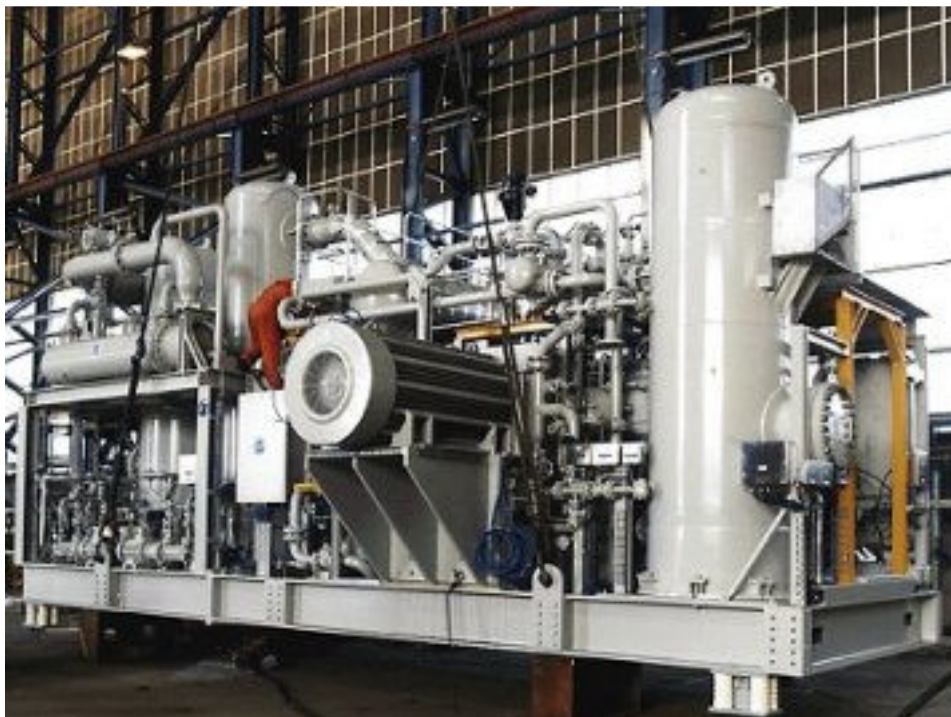
Figure 1: Flare gas compressor package for a FPSO in the North Sea
