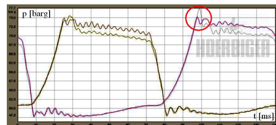
Figure 3: p-t traces at two different times laid onto each other reveal a sharp pressure rise (grey curve) at the discharge valve opening hinting at oil sticktion [1]
