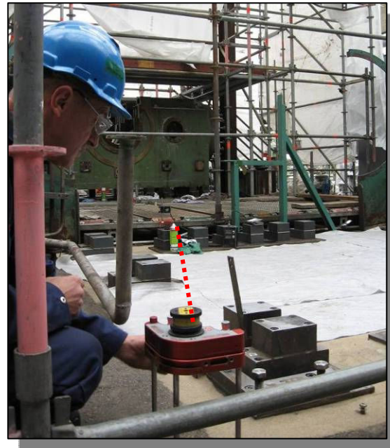
Picture no. 6: Laser Planarity Check
