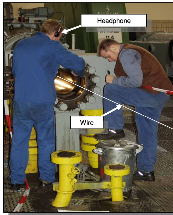
Picture no. 19: Alignment through Steel Wire
