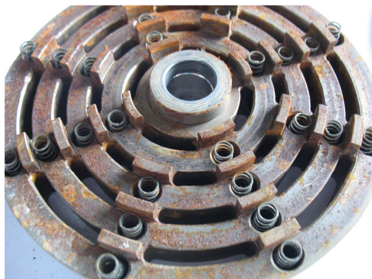
Figure 25: Internal parts of a CC valve
