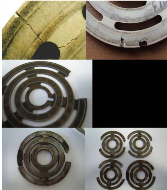
Figure 1: Typical failure modes of standard valve plates in high speed compressors
