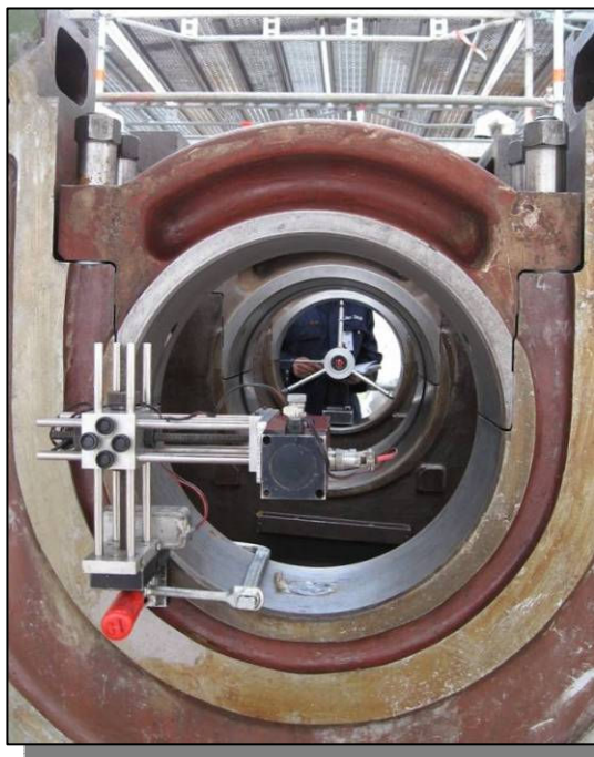
Picture no. 9: Bearing Way Alignment Check
