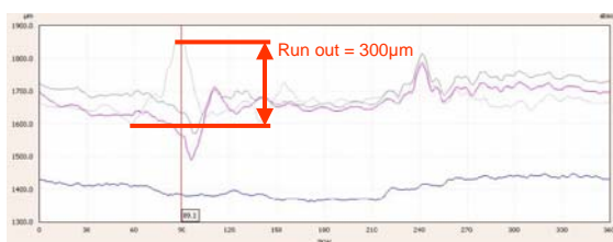
Figure 12: Run-out as function of crank-angle; 30 minutes after first failure indication
