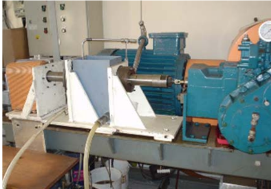
Fig. 6: Test rig for performing measurements of the frictional forces acting in the counterfaces of packing and cylinder rings
