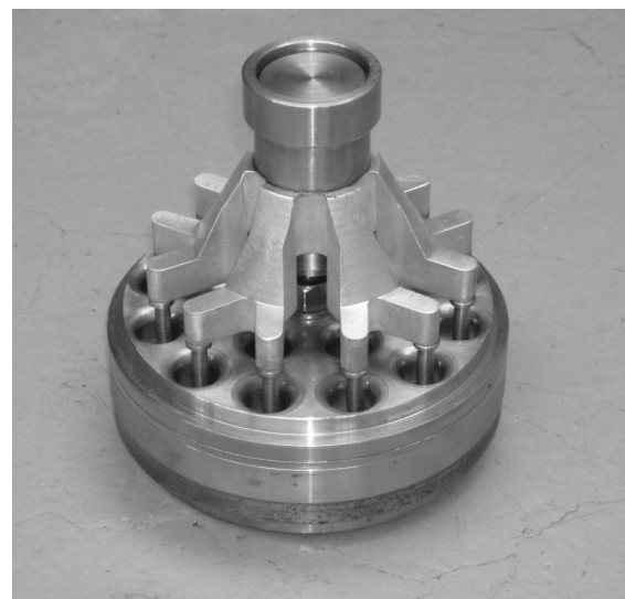
Figure 12: Unloader for the Burckhardt poppet valve TM
