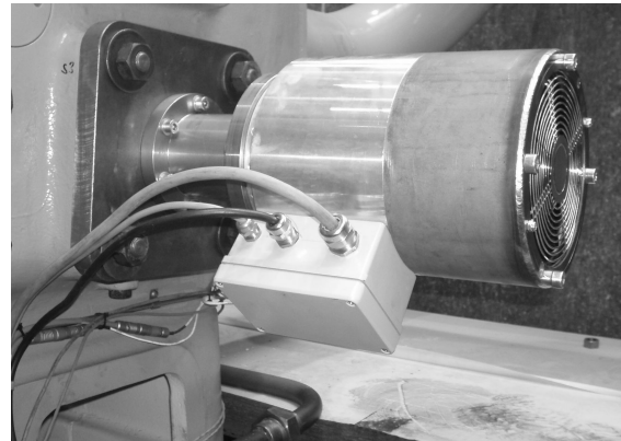
Figure 19: Capacity control mounted on a two stage test compressor
