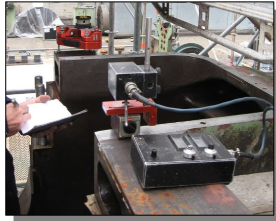
Picture no. 10: Frame Top Planarity Measurement
