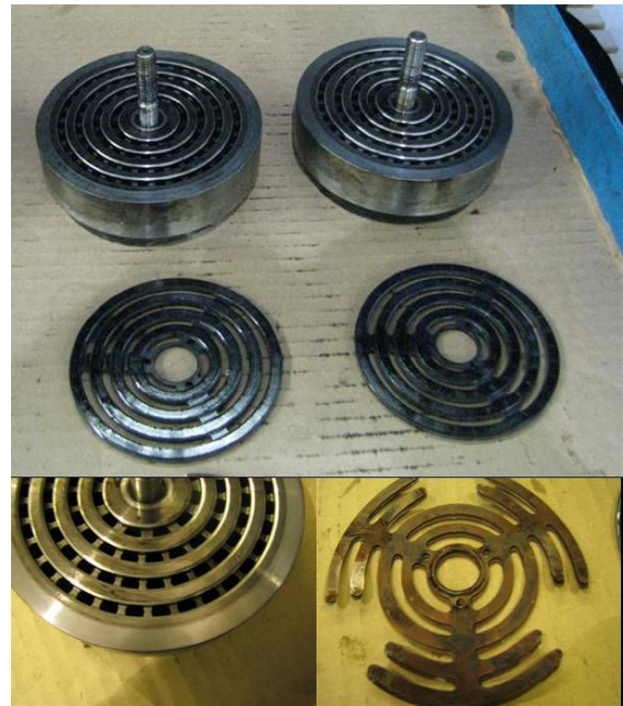
Figure 12: Valve inspection of a 90CPs valve after 5000 hours of operation in demanding gas gathering installation in Canada
