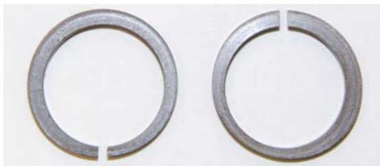
Fig. 3: Non-uniform wear pattern of a cylinder ring pair
