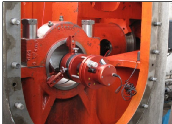
Picture no. 29: Transmitter Fixation at Bearing Block
