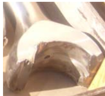
Figure 20: Fractured con-rod small end
