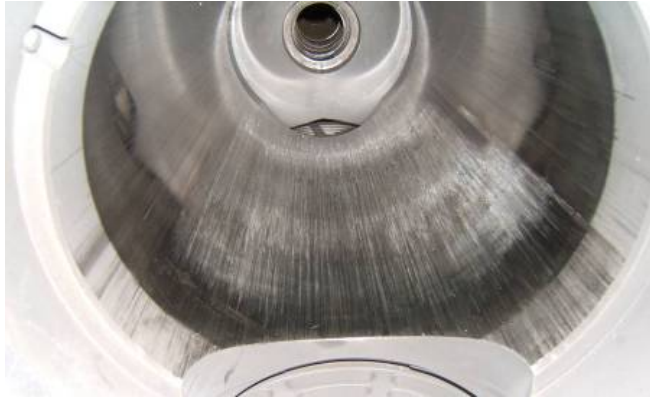
Figure 1: Damage to liner, rider ring wear not detected
