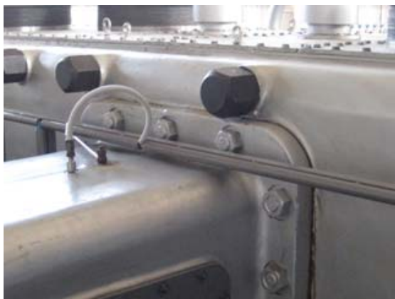
Figure 1: Accelerometer to measure high-frequency vibrations mounted on crosshead slide
