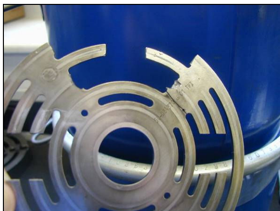
Picture no. 10: Broken valve plate 6 th stage
