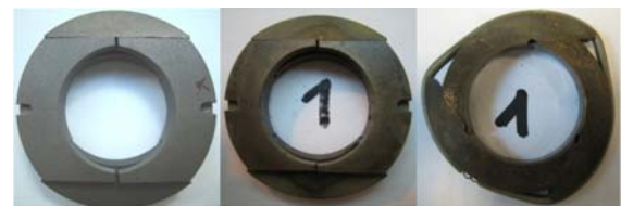
Fig. 10: Back views of virgin BCD ring (left-hand), worn BCD ring (middle), and worn tangential cut ring
