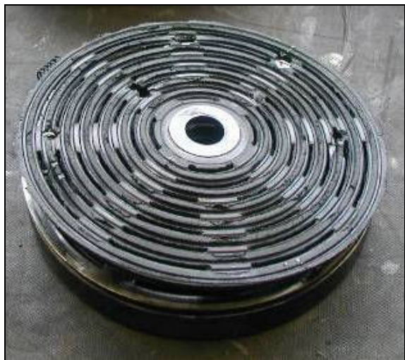
Picture no. 9: Holes in valve plate 5 th stage
