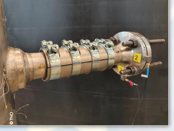
Experiments at TNO in Delft to find an efficient solution for a common problem at reciprocating compressor installations - Preventing vibrations at Small Bore Connections (SBC) by the use of visco-elastic layers.
